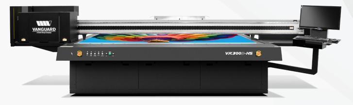
The VK300D-HS printer is a part of our 7-time award winning VK Series. It is a fully featured printer that has revolutionized the industry with a high-speed electromagnetic drive system that propels the carriage at speeds up to 1.8 m per second for an incredible up to 317 m<sup>2</sup> an hour.
