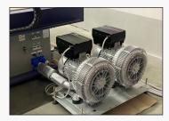
Equipped with two 5.5 kilowatt blower motors for maximum substrate stability while printing.
